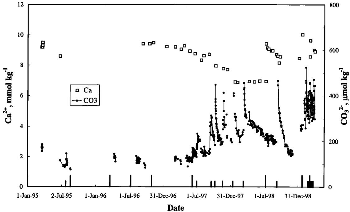
**Figure 1.** Time series of  $\text{Ca}^{2+}$  and  $\text{CO}_3^{2-}$  concentrations. The short vertical bars along the ordinate indicate when  $\text{HCO}_3^-$  and  $\text{CO}_3^{2-}$  were added, and the long bars indicate when  $\text{Ca}^{2+}$  was added.
