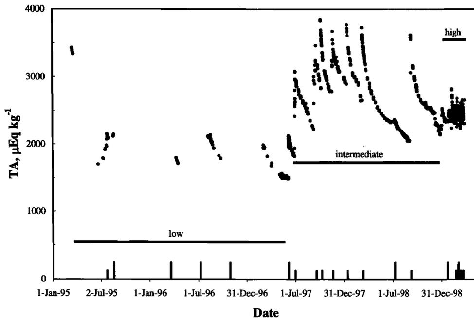
**Figure 2.** Time series of total alkalinity (TA). The horizontal reference lines indicate the step changes in saturation state. The vertical bars along the ordinate denote when and what type of chemical addition occurred as explained in the legend for Figure 1.
